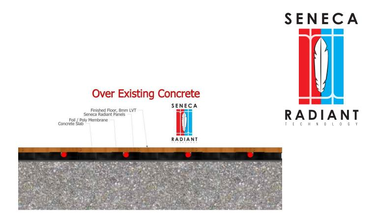
Determine the amount of panels and tubing required, calculate the area to be radiant heated. Each radiant panel requires 2-feet of radiant tube. Provide enough tube to reach the manifold assembly or main supply piping.
